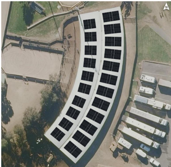
FIGURE 10: AELEC – 134-kW SOLAR ON CATTLE HOLDING AREA W/ 120 kWh BESS
