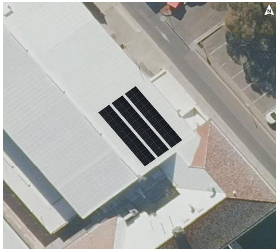
FIGURE 23: TOWN HALL – 15 kW SOLAR ON THE NORTHEAST-FACING ROOF
