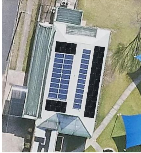
FIGURE 41: BARRABA POOL – 10.5 kW SOLAR ON THE ROOF AREA ON THE POOL SIDE ADJACENT ROOF SPACES NEAR THE CURRENT INSTALLATION W/ 30 kWh BESS
