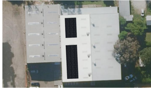
FIGURE 91: 7-11 ANNE STREET – 40.5 kW COMBINED SOLAR SYSTEM (25.5 kW FOR INFLATABLE WORLD AND 15 kW FOR TAMWORTH BOULDERING)
