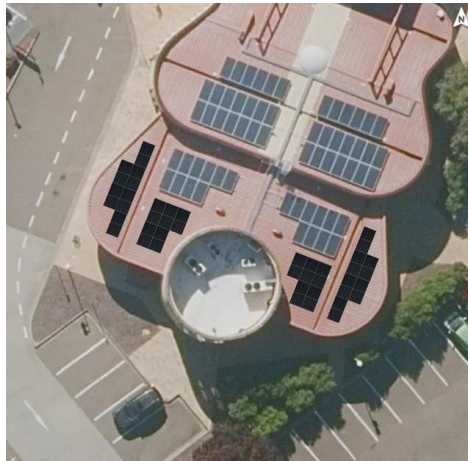
FIGURE 35: AUSTRALIAN COUNTRY MUSIC HALL OF FAME – 13 kW SOLAR ON SOUTHEAST AND WEST ROOF SECTIONS W/ 6.4 kWh BESS
