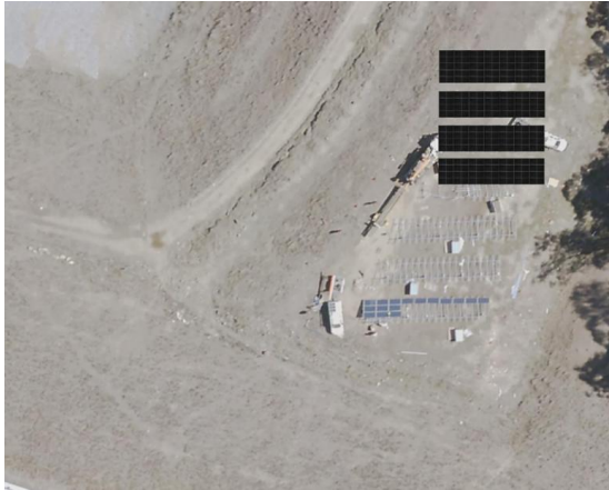
FIGURE 58: DUNGOWAN DAM – 71.4 kW GROUND-MOUNTED SOLAR PV SYSTEM ABOVE THE CURRENT SYSTEM W/ 230 kWh BESS
